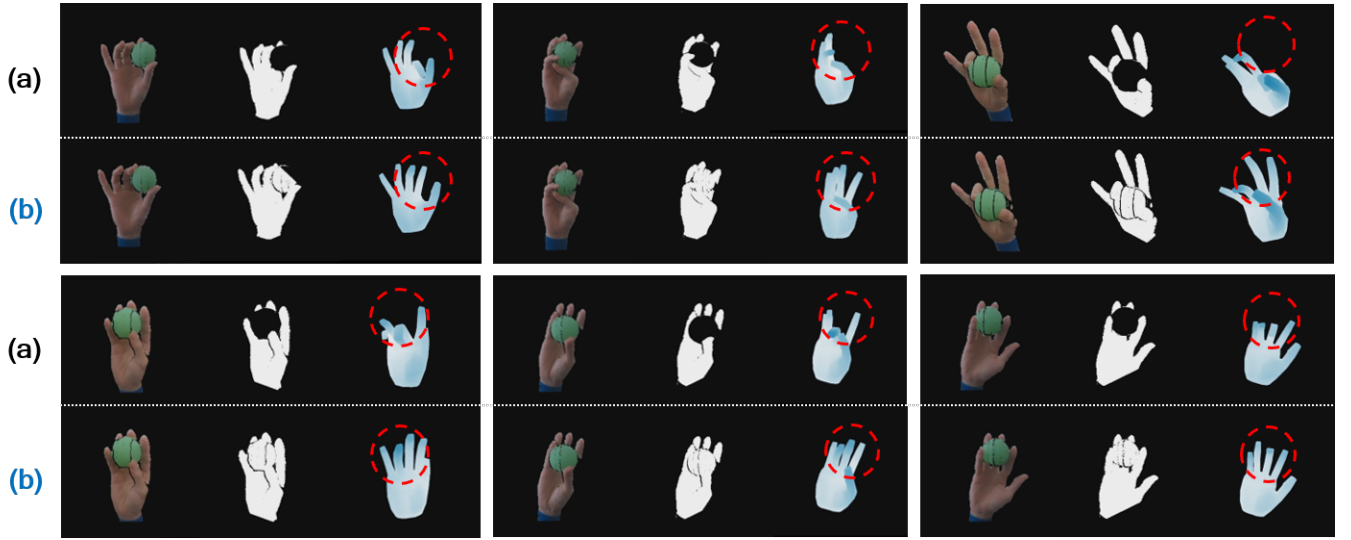
Figure 3: Self-Qualitative comparison. Each image set shows, RGB image(1st column), depth image(2nd column), estimated pose(3rd column). (a) Without depth reconstruction (b) With depth reconstruction
