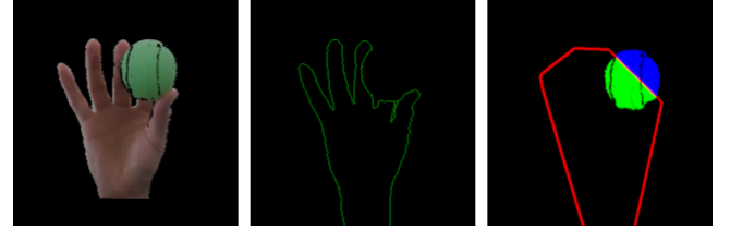
Figure 2: Reconstruction area(Green). RGB image(Left), Contour(middle), Convex hull(right).
